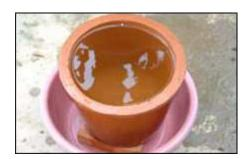
When tests are complete the pots are coated inside and out with colloidial silver to add an additional protective bacterial killing component.
