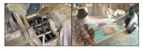
These two ingredients (18% rice, 82% clay) are mixed with water in a modified mortar mixer then kneaded into 10kg pieces.
