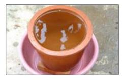
When tests are complete the pots are coated inside and out with colloidial silver to add an additional protective bacterial killing component.
